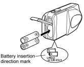
There is a mark showing the correct way to insert the AA batteries on the bottom of the camera
