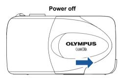
TIP To maximize battery life, the Digital camera features a power saving mode in which the camera enters a sleep mode after approximately three (3) minutes of non-use.
