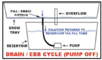
Figure 3. The Ebb and Flow System.
