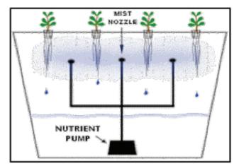
Figure 6. The Aeroponic System.
