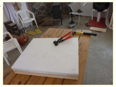
heavy duty pliers with a wide gripping head. A little practice with a hand seamer and you'll be making sheet metal bends like a pro!
