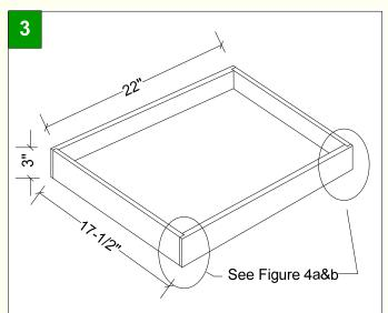
The sides of the telescoping cover is a simple frame. You can use either a simple butt joint (Figure 4a) or a rebate joint (Figure 4b) to minimize exposed end grain.
