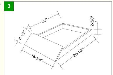
Compared to a conventional hive stand, a hive stand for an IPM bottom board has a wider landing board and a slightly different profile of the side rails.
