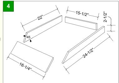
From 1x4 cedar or pine ripped to 2-1/2" wide, cut two sides 24-7/8" long and one back piece 15-1/2" long. Make a 45-degree angled cut on the front of both side rails. From a 1x6, cut a 16-1/4" piece for the landing board.
