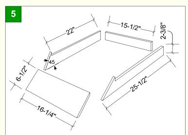
For the IPM Bottom Board version, from 1x4 cedar or pine, cut two pieces 25-1/2" long and one back piece 15-1/2" long. From a 1x8, cut a 16-1/4" piece for the landing board.
