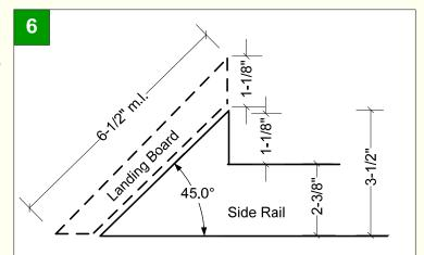
Detail of the side rail for the IPM Bottom Board version. Using a full width 1x4 cedar or pine, make a 45-degree angled cut at the front. Where this angle meets to top, measure down 1-1/8" and then remove a strip of this depth to the end of the rail. When mated to the landing board, the total depth from the top of the landing board to the top of the side rail will be about 2-1/4".
